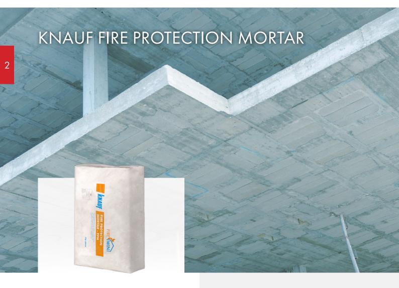
Knauf Fire Protection Mortar is a dry white powder consisting of inorganic compounds and perlite. When mixed with water the compounds form a highly thermally insulating fire seal to prevent the spread of fire and smoke through openings in fire rated walls and floors, including openings formed to accommodate building service penetrations.
